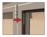
Lastly pack the top side corner on the hinge side of the door. Use a variety of packers until the glazed unit sits firm in place. This will help keep the glazed unit square and in place.
