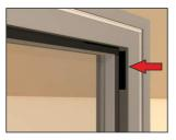
Pack the side of the unit on the handle side of the door. Use a variety of packers until the glazed unit sits firm in place and square within the frame.
