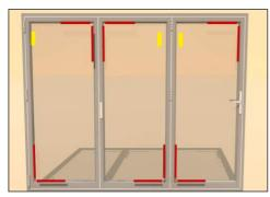
The red sections display where to toe and heel on a 3 panel door all one way.
