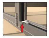
Place 2-3 packers at the bottom of the door on the hinge side.
